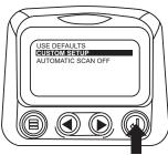
10. Use the "Arrow Buttons" to scroll to and highlight a selected parameter (parameter with a # symbol to right of it).
